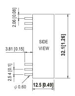
NOTE: Pin tolerance ±0.05mm
