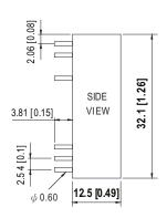
NOTE: Pin tolerance  $\pm 0.05$ mm
