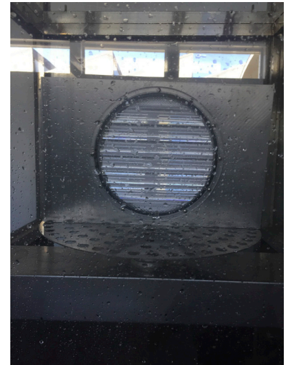
Test Under Water Jet
